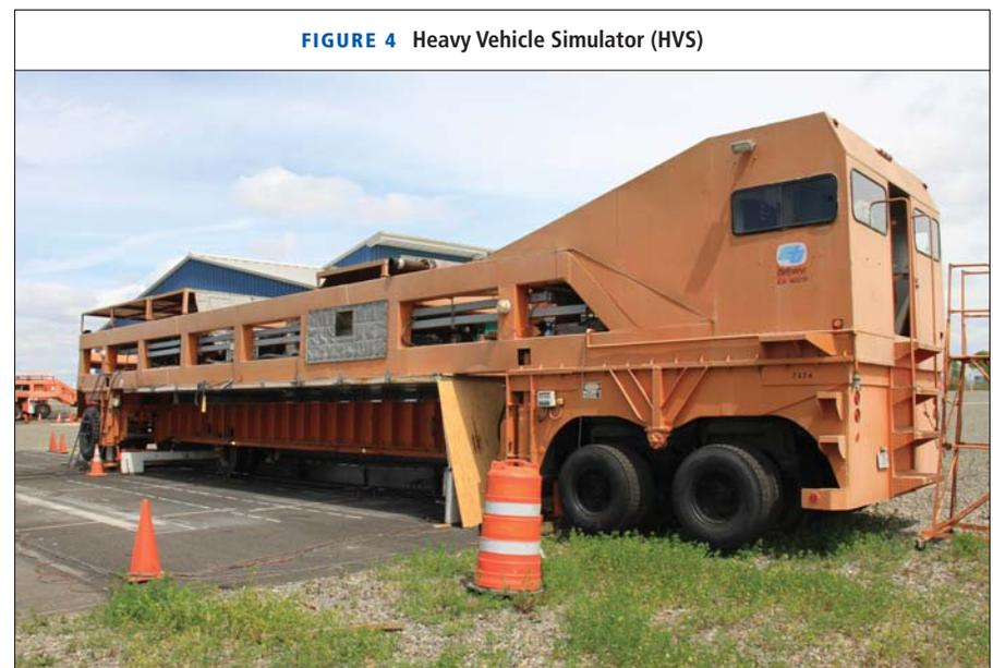
**FIGURE 4 Heavy Vehicle Simulator (HVS)**
