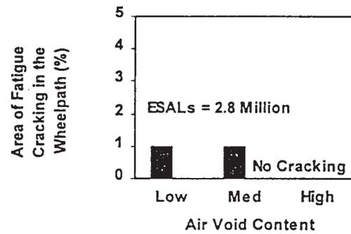
*Fine plus gradation at optimum asphalt binder content*
