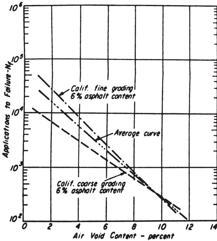
Figure 6. Influence of air void content on fatigue performance
