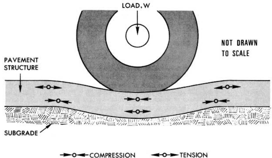
Figure 2: Pavement deflection results in tensile and compressive stresses in pavement structure.
