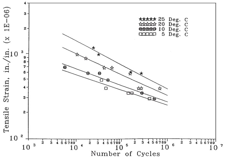
Figure 5. Strain-versus-fatigue relations for different temperatures
