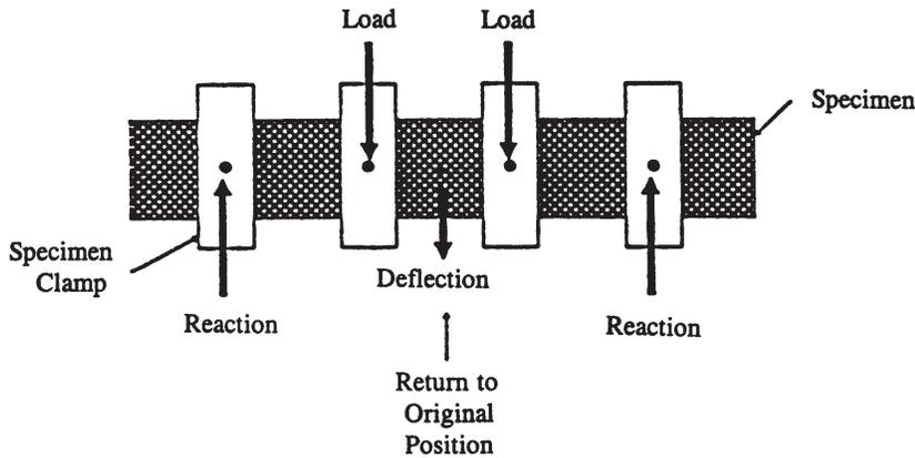
Figure 4. Schematic of third-point loading fatigue test apparatus
