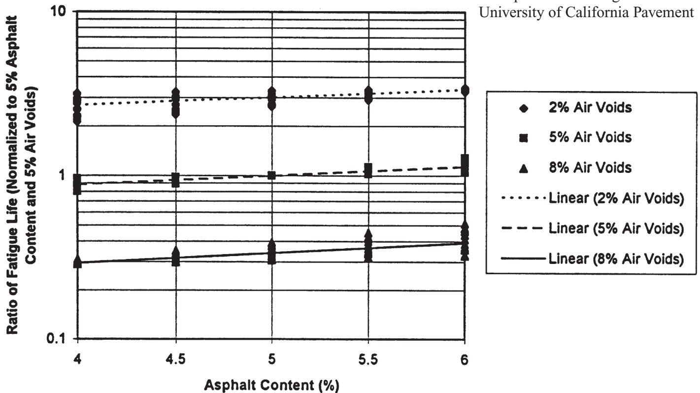
Figure 7. Effect of asphalt and air-void contents on simulated, fatigue-life ratio for 270 mix-pavement combinations
