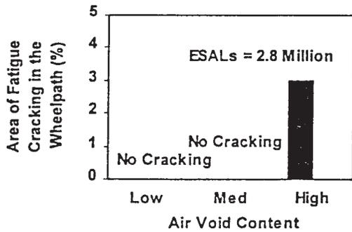
*Fine gradation at optimum asphalt binder content*
