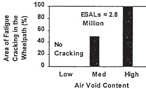
*Coarse gradation at optimum asphalt binder content*
