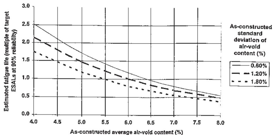
Figure 3. Effects of as-constructed air-void content on pavement fatigue performance (chart from TM-UCB-CAL/APT-97-1)
