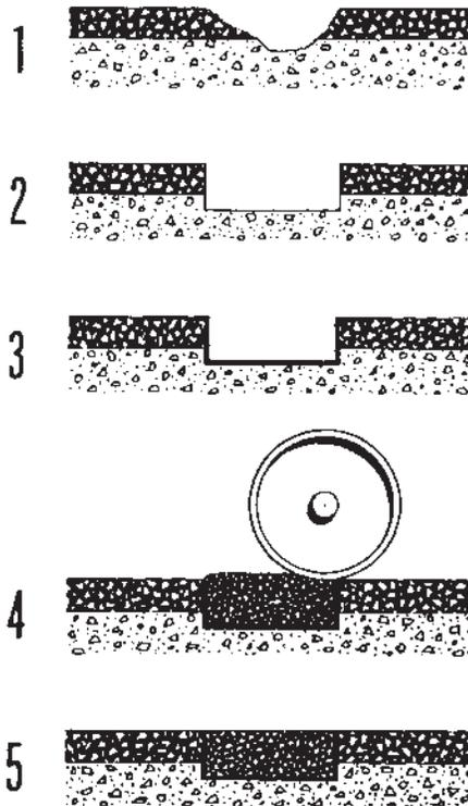
Figure 6. Pothole permanent repair (courtesy The Asphalt Institute)
