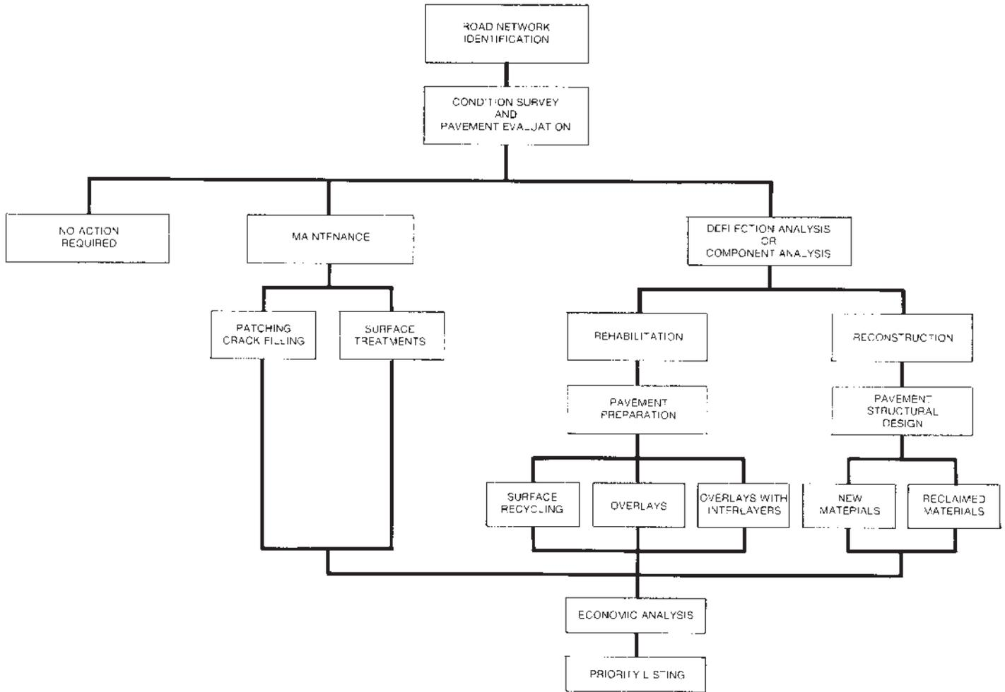
Figure 4. Plan-development guide (courtesy The Asphalt Institute)
