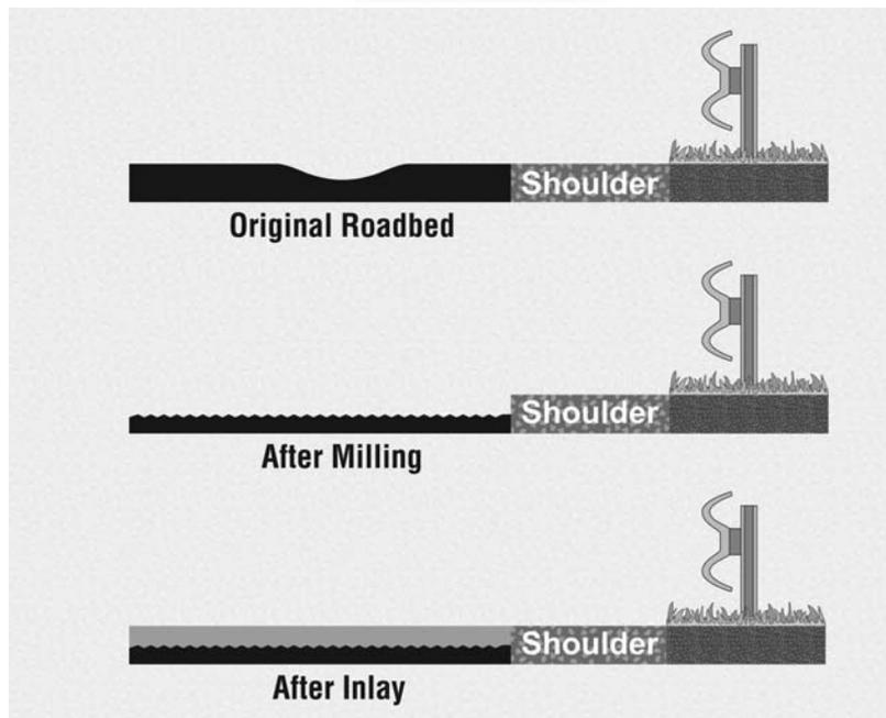
Mill and Fill Process Eliminates Need for Shoulder and Guardrail Changes
