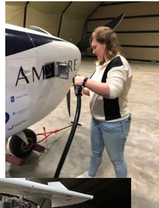
Plugs directly into aircraft front cowling (SAE AS6968)
